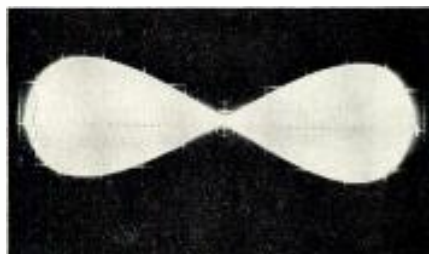
Fig. 2. Bow-tie monitoring with 19-kc sine wave (pilot subcarrier) on shown X-axis.
