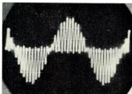
Fig. 1. Monitoring composite signal with internal sweep synchronized on the audio.
